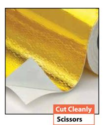
Gold Foil is made from lightweight aerospace material. This 6 mil thick foil has a fire resistant pressure sensitive adhesive that incorporates a fiber-glass backing for strength and tear resistance. The adhesive meets or exceeds the FAA 12-second vertical burn requirement.
