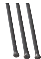
Comparison of monofilaments: flat versus round (magnified for better visibility)
