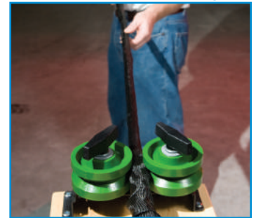
4. Pull Wires & Sleeving
